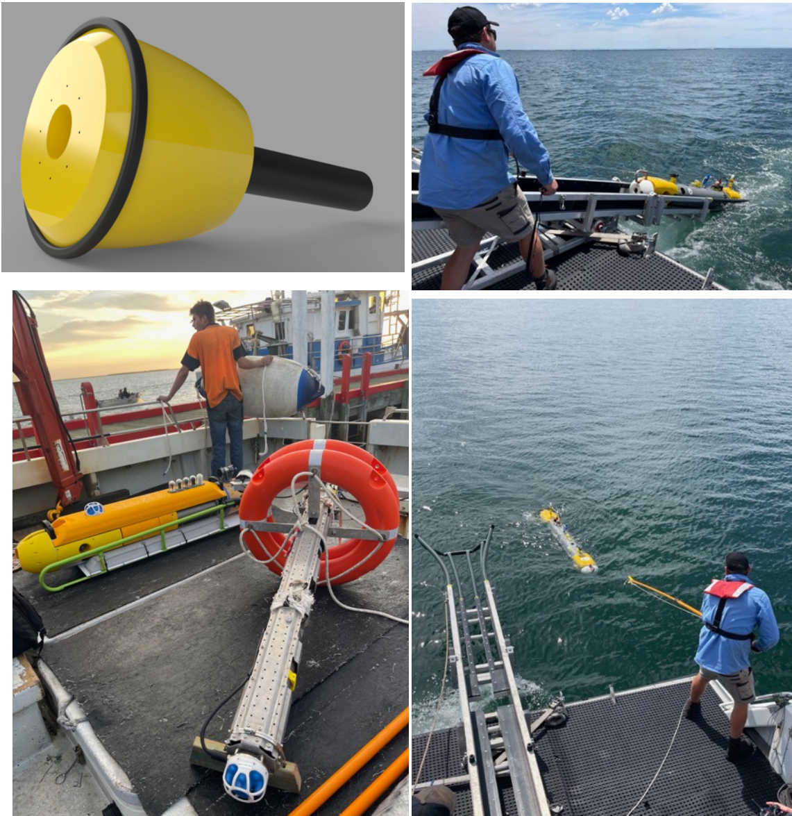
Figure 1. Example AUV operational elements. Clockwise from top left – Diagram of surface tracking buoy to be used for campaign, previous generation of AUV being hauled up the Launch and Recovery system (LARS), previous generation of AUV being hooked for recovery up the LARS, surface tracking buoy prototype showing surface satellite receivers and USBL pole along with the Seeker class AUV that will be used for Bass Trek campaign.
