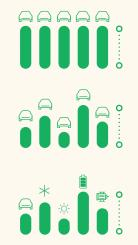
**Balanced -** All chargers are ramped up and down at the same time. Responding to the overall site electrical capacity.
