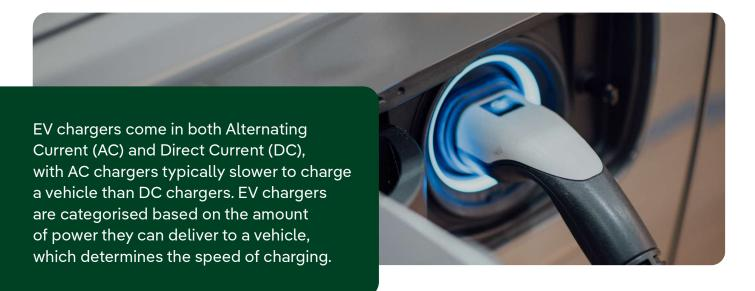
The slowest charging rate would be through a wall socket that supplies 2kW and charges a typical passenger vehicle in 35 hours. The fastest chargers are 350kW DC chargers that can charge a typical EV in 30 minutes.
